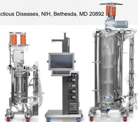
Figure 4. HyPerforma eS.U.F. 30L and 300L Vessels with TruBio Controller. The volume used would depend on the site scale needs.
